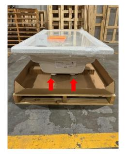
Our boxing process beings with a pallet and box bottom before setting the tub on to the box bottom. Next, we install 3" adhesive runner that serve two purposes;
